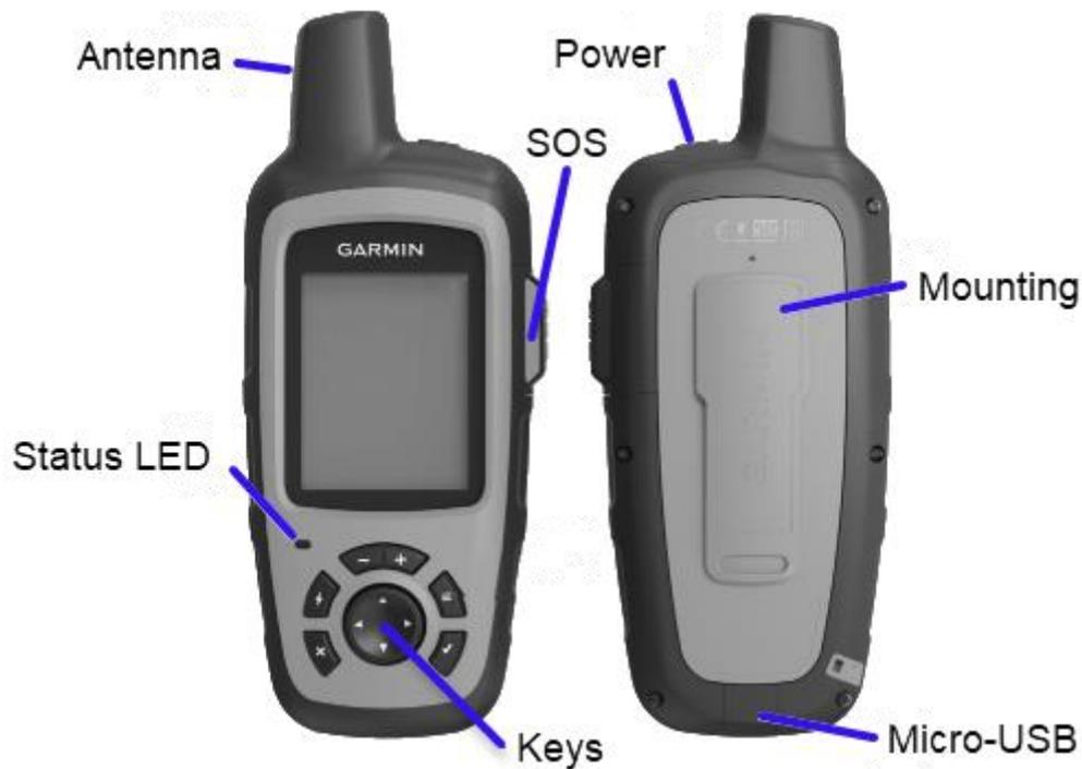
**Antenna:** Keep the satellite communicator antenna pointing up toward the sky and the face of the device pointing away from your body.
